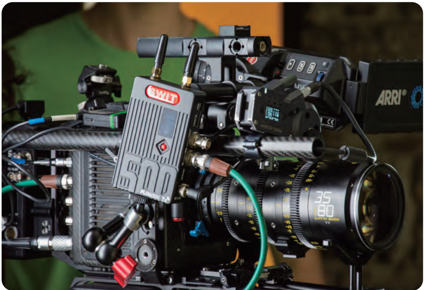
The 150m wireless SDI transmitter on ARRI ALEXA MINI LF setup, for professional cinematographers. Model: FLOW500 (Tx), Page 15.
