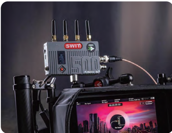
The 150m wireless SDI receiver for handheld mobile monitoring. Model: FLOW500 (Rx), Page 15.
