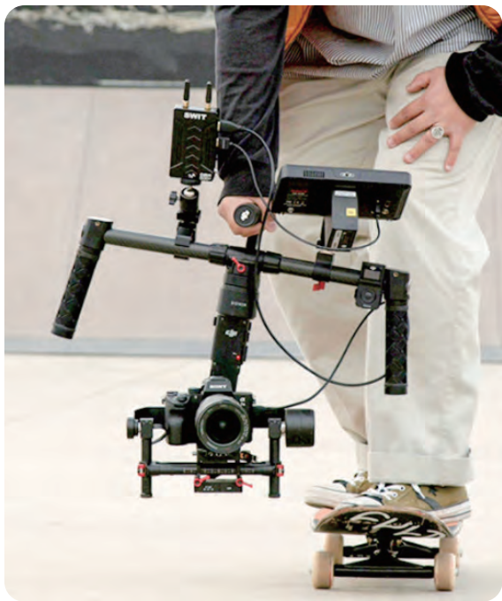
The 150m wireless HDMI transmitter on DJI. Model: CURVE500+ (Tx), Page 15.
