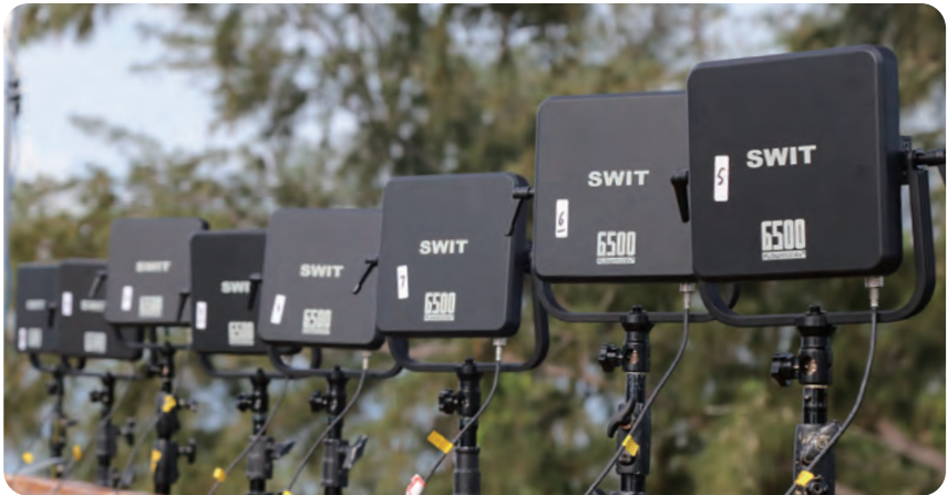
The 2km long range wireless SDI receivers, up to 22 camera channels working wirelessly together, no interference to each other. Model: FLOW6500 (Rx), Page 16.
