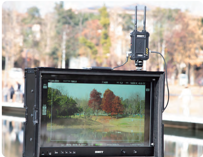
The 1.2km wireless SDI receiver working on site for director monitoring. Model: CREW (Rx), Page 14.
