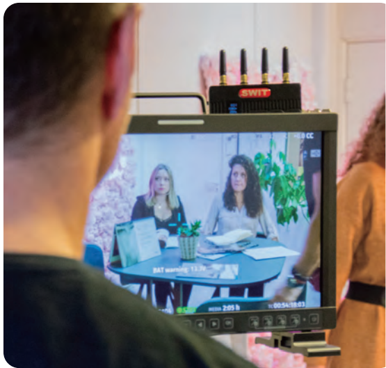
The 150m wireless SDI receiver. Model: FLOW500 (Rx), Page 15.
