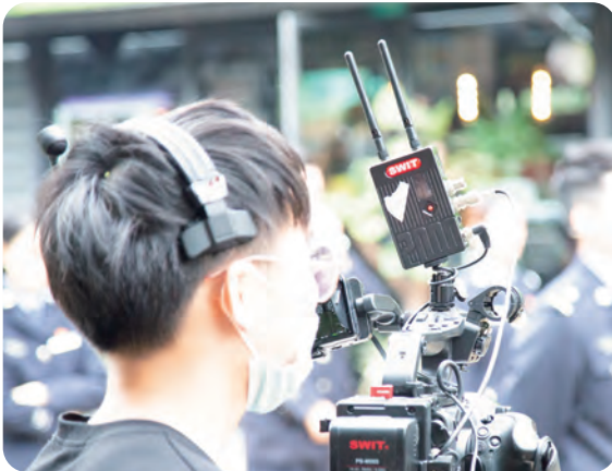
The 600m wireless SDI transmitter on SONY FX6 camera for live production. Model: FLOW2000 (Tx), Page 15.
